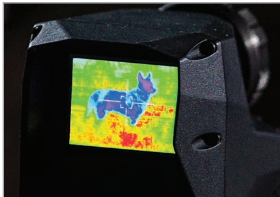
The Display View with LCD Color for Day/Night Time Direct View Targeting.
